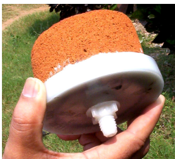
100 mm diameter Terafil water filtration disc fitted with food grade plastic holder
